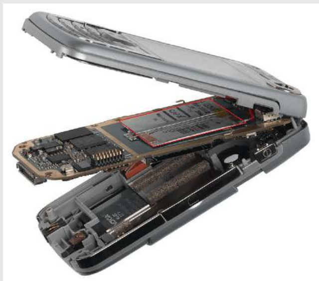
Cutaway image of a cellular phone showing the interior components, many of which contain and depend on minerals and mineral products to function. SOURCE: CAP-XX Ltd.
