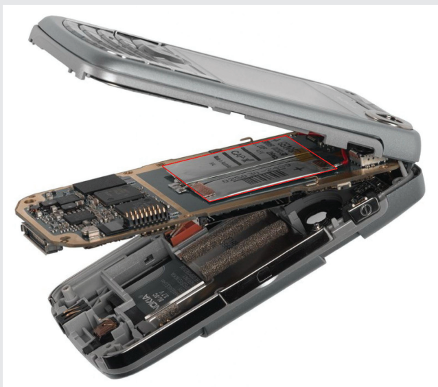
Cutaway image of a cellular phone showing the interior components, many of which contain and depend on minerals and mineral products to function. SOURCE: CAP-XX Ltd.
